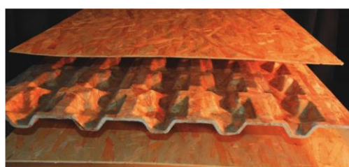
Figure 1: Wood-strand sandwich panel with 3-D core.
