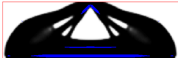
Figure 1: Optimized layout of a simply-supported reinforced concrete deep beam subject to a point load. Black = concrete; white = void; blue lines = rebars.
